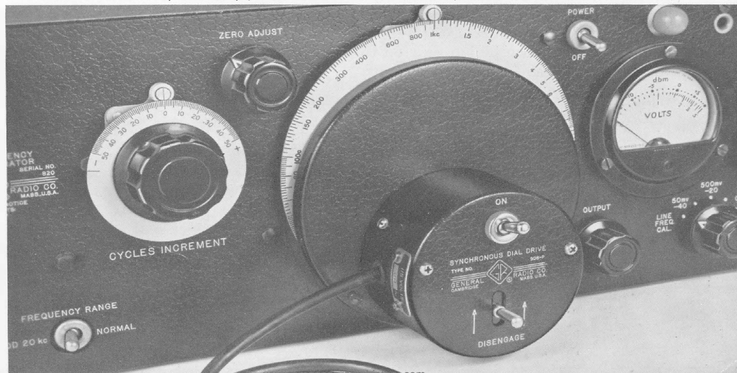
Figure 1. View of the Type 908-P2 Synchronous Dial Drive installed on a Type 1304-B Beat-Frequency Oscillator. The adjustable stops, which attach to the oscillator dial, are not shown.
